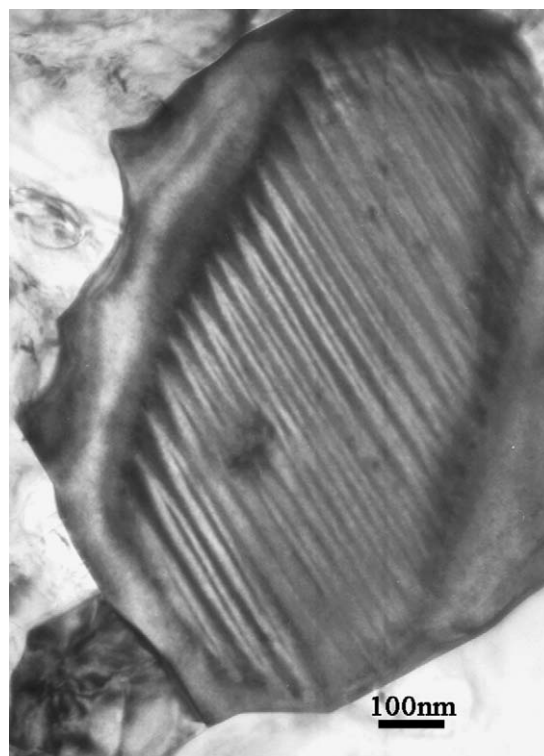
Fig. 5. TEM micrograph of HDK[C] ceramic showing the core–shell structure.
